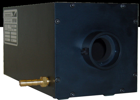
CL7 Enclosed UV Spectral Irradiance Standard 200-400nm
